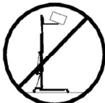
**3.4** - This lifter should NEVER be used to elevate a load that has not been properly checked. It is necessary to verify that the load is correctly supported and centred on the appropriate lift support so that the weight of the load will only elevate in a vertical direction.
