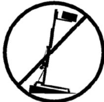
**3.2** - Only place the lift on hard, flat surfaces always checking that it is in a vertical position by using the bubble level indicator found on the base. Adjust the leg stabilizers by turning the handles to level if necessary. NEVER use wedges or other foreign objects to balance the lift.
