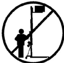
**3.8** - NEVER move the lift whilst it is carrying a load and elevated over 2.5m. It is not advisable to carry out any type of horizontal movement even small positional adjustments. You can only move the lifter when is load at **minimum** height.
