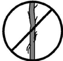
**3.12** - Before using the lift, check the condition of the cable. The cable should not have broken threads or show any signs of crushed/flattened areas. NEVER use faulty cables, always change them if there is any doubt. Only use Kuzar Industrial steel cables; reference: DIN 3060. Quality: 180KG/mm and torsion resistant.
