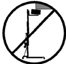
**3.10** - Be careful with all obstacles above the lift and its extension zone such as cornices, balconies, and luminous signboards. It is very important to avoid the presence of all types of cables below the extended lift.
